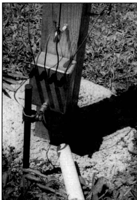
Figure 3—Near the base of the center pole, an aluminum enclosure houses the four relays. The four wires from the top of the pole are anchored at the pole base in large eye bolts, one on each face of the pole. Each wire's bottom end connects to the inside of the relay box through binding posts. From the hidden pole face, the wire passes through a hole drilled in the pole near the eye bolt above the relay box. The feed line approaches the pole through a piece of PVC pipe and is attached to the box via a BNC connector. A ground rod connected to the relay box finishes the installation.
